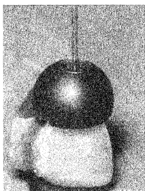
Figure 6. Steel hemisphere attached to approximal surface with pin shaft extending through center channel; the 3 mm diameter of the center channel allowed the load to be applied with only approximal enamel (not the restoration) supported by the hemisphere.
