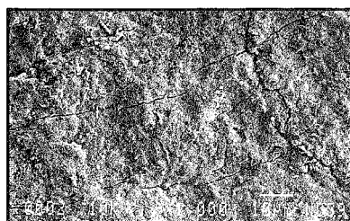
Figure 4. SEM photograph of fractured alumina air-abraded specimen after the tensile bond test. Cohesive fractures of enamel were observed on the enamel side (original magnification X500)
