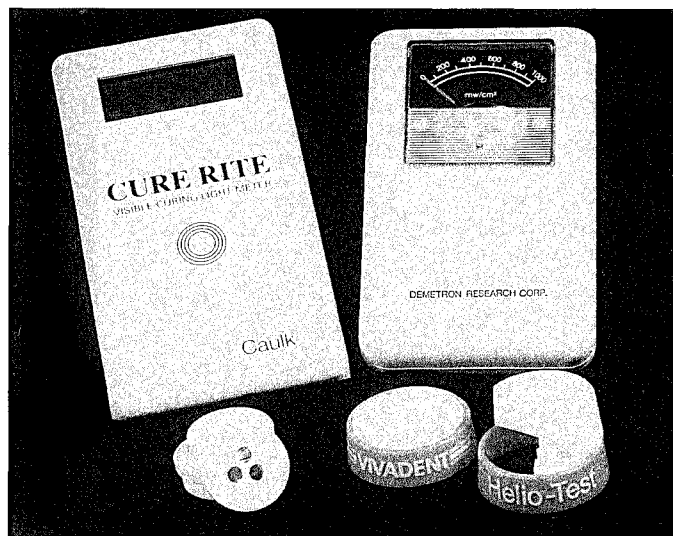
Figure 5. Radiometers, hardness disks, and split resin molds used in the monitoring of light-curing unit output
