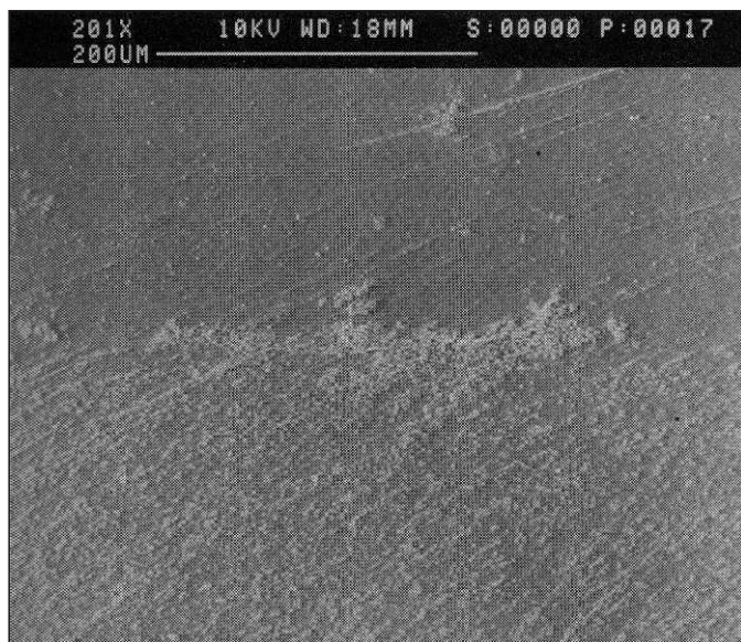
Figure 3. Marginal imperfection: Any kind of incontinuity of the restoration/tooth (enamel or dentin) interface but no marginal gap, eg, overhang or underfilled margin (201x magnification).
