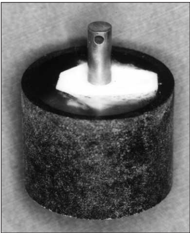
Figure 1. A specimen for measuring tensile bond strength.
