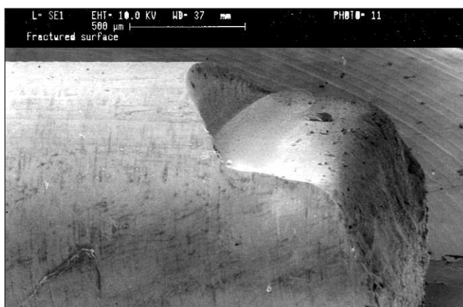
Figure 5. SEM photograph of a fractured ceramic post.
