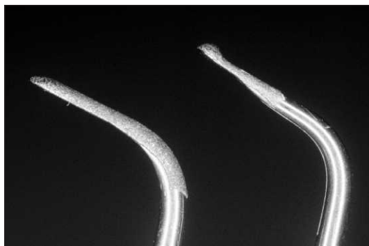
Figure 2. One-side coated diamond instruments for use in oscillating handpieces (Sonic Sys, KaVo, D-88400 Biberach, Germany).
