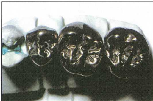
Figure 8. (left) Partial veneer castings after investment removal with acid. These castings have not been polished and will need very little polishing because of the fine surface finish and the accuracy of the laboratory investment and casting procedures.
