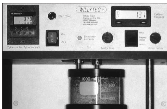
Figure 4. ACTA-machine with the sample wheel in a millet seed suspension.
