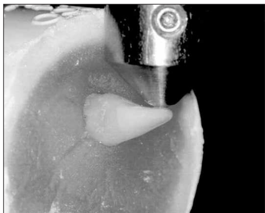
Figure 3. Load testing at 90° degrees with Instron Universal Testing Machine.
