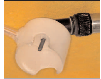
Figure 4: Device ready for use. Sandblaster attached to the top small hole and bottom concavities for best fitting in the working area.
