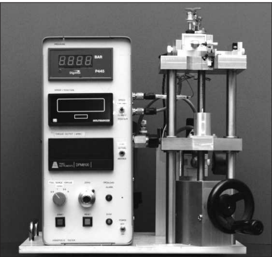
Figure 1. General view of the front of the prototype handpiece testing machine. The load frame is on the right, with the test stations on top, and the electronics on the left, with the displays of air pressure, speed and torque.
