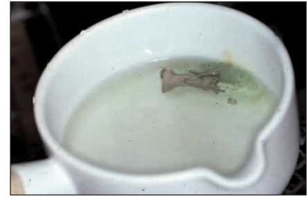
Figure 7. Example of dissolving nickel silver posts with warm concentrated nitric acid.
