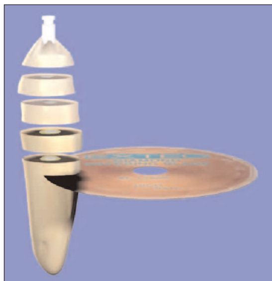
Figure 1: Perpendicular sectioning of root-post sets into approximately 1-mm thick sections.
