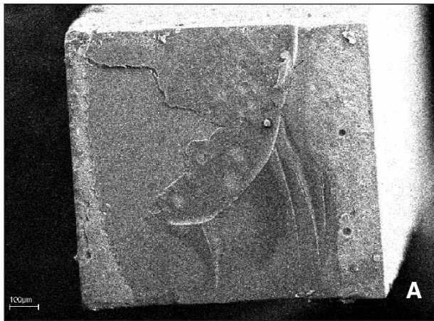
Figure 1. SEM images of the fractured dentin surface of a specimen bonded with Single Bond after cyclic loading. Figure 1A) A mixed failure may be observed, with resin composite present at the right and left margins and adhesive in the central area. Figure 1B) A higher magnification view of the failure that occurred at the top of the hybrid layer.
