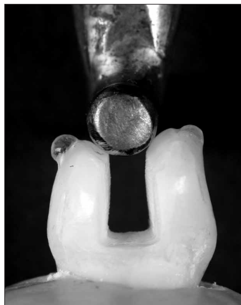
Figure 2: Premolar with MOD cavity preparation, showing both the loading cylinder in contact with the cuspal inclines and the glass balls fixed at 0.5 mm from the cusp tips.
