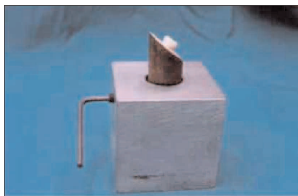
Figure 5. Attachment holding the ring with mounted specimen at an angle of 45°.
