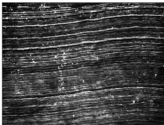
Figure 3C: Herculite XRV surface with varying roughness after the use of two diamonds.
