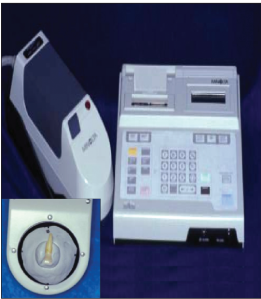
Figure 1: Minolta Chroma Meter CR321 with PVS jig and sample tooth in place.
