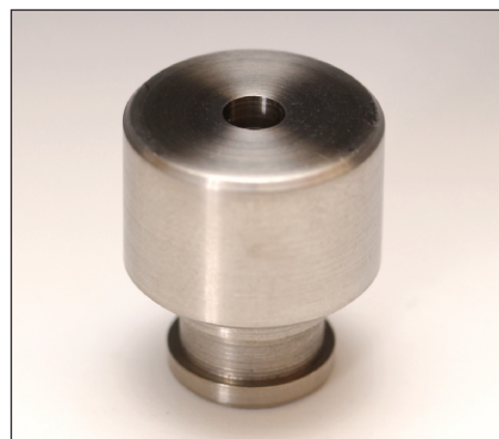
Figure 2. Stainless steel custom fixture for resin composite specimen.
