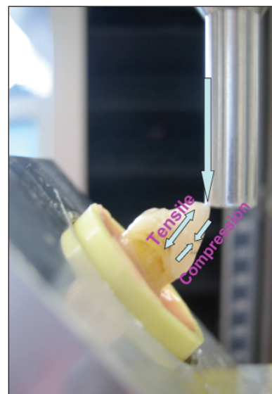
Figure 1: Application of the load cell to the laminate-tooth interface until fracture in a universal testing machine.
