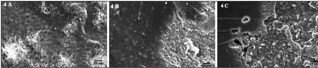
Figure 4: SEM of fracture dentin surfaces treated with Prime & Bond NT adhesive system. Figure 4A applied according to the manufacturer's instructions, Figure 4B doubling the number of adhesive layers followed by curing, Figure 4C doubling the number of layers with intermediate curing.
