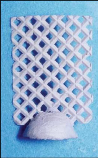
Figure 2. Casting produced to evaluate castability of the Duralay pattern. A rectangular-shaped matrix was evaluated for the number of diamonds cast.
