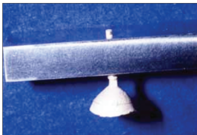
Figure 5. The dimensional stability casting is placed back into the stainless steel pattern former to evaluate casting and dimensional changes from the original Duralay pattern. The casting passes through the pattern former, indicating shrinkage in the size of the pattern.
