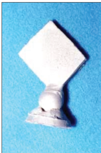
Figure 3. Casting produced to evaluate the surface roughness of the casting. This is a square pattern measuring 1.5 cm in length, made against a glass slab.
