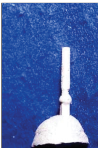
Figure 4. Casting produced to evaluate dimensional stability. This casting is produced from a 10 mm pattern that is 2.5 mm wide at the base and 2.0 mm wide at the apex. This produced a tapered casting.
