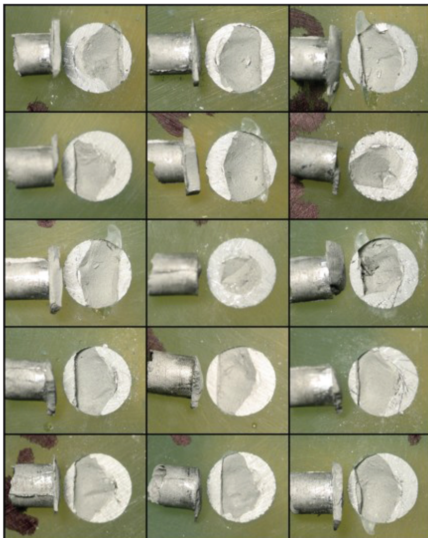
Figure 6: The 15 specimens from the two-month (70 day) sample shown in sequential order with their fractured columns alongside, all exhibiting C1 cohesive type fractures.
