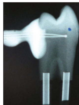
Figure 2. Radiograph of a tooth with a temperature sensor.
