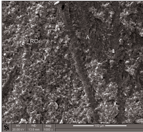
Figure 2. Representative SEM micrographs of the dentin side of a fractured beam from the ARC-tungsten carbide group. Mixed failure involved adhesive failure at the composite-cement interface and cohesive failure between the adhesive and cement. The resin cement was found laying on top of the fractured adhesives. RC: fractured resin cement; A: fractured adhesive. (Original magnification = 1000x)
