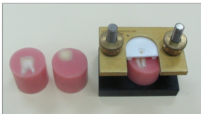
Figure 1. Utradent mold setup for the shear bond strength test (left: axial dentin surface; middle: occlusal dentin surface; right: Utradent jig setup on the axial dentin surface).
