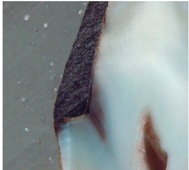
Figure 1. Longitudinal Section Showing Silver Nitrate Penetration.
