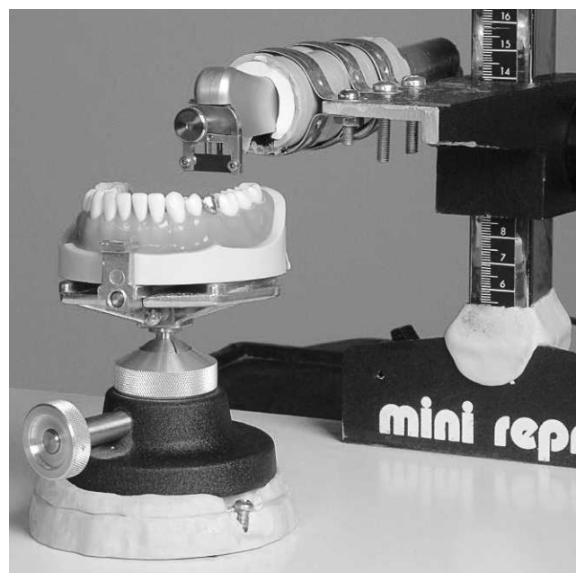
Figure 2. Custom-made setup to standardize measurement using the Tooth Pressure Meter
