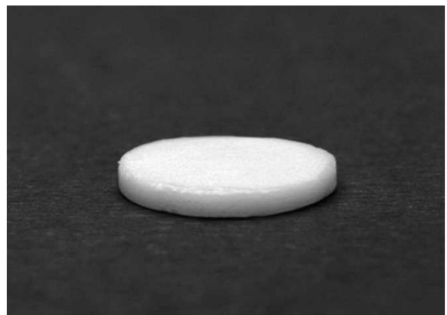
Figure 1. Ceramic disk 1.5 mm thick and 12 mm in diameter.
