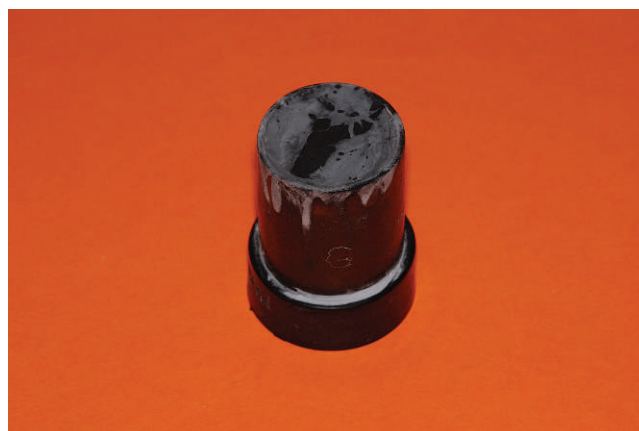
Figure 13. Patterns are invested in the casting ring using 15 cc of water and 50 g of investment (Novacast, Whip-Mix Co, Exeter, KY, USA) for maximum expansion. Castings are cut from the sprue but not finished. The sprue remnant is reduced with a small diamond point after cementation when the cement is set.
