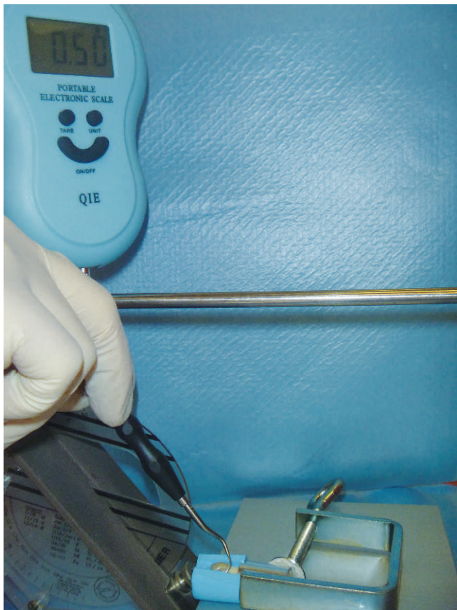
Figure 3. Dynamometric appliance used to standardized the force and the direction of the strokes.
