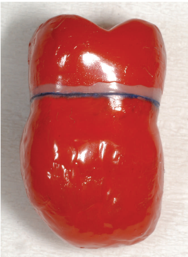
Figure 5. Specimens covering and margin exposure for microleakage test.
