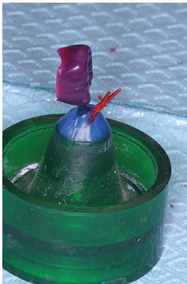
Figure 10. Wax-up and plastic burnout pins on sprue former.
