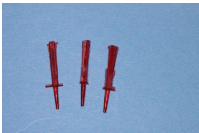
Figure 8. Plastic burnout pins used for vent pin.
