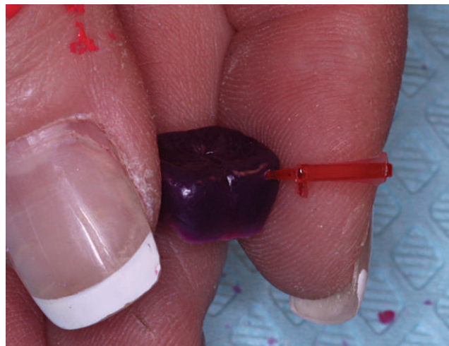
Figure 9. View showing plastic burnout pin in hole created in wax. The mesio-buccal usually is the best place to place the escape channel since it is easily accessible for finishing.
