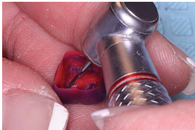
Figure 7. Handpiece carefully making hole in wax pattern—a small twist drill can also be used for this step. It is important that the hole must be the size of the plastic burnout pins seen in Figure 25.
