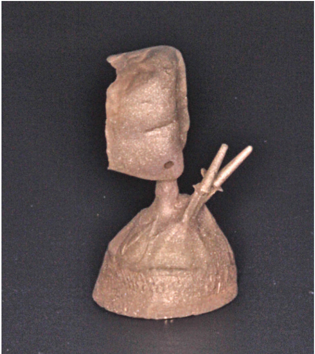
Figure 11. Casting following pickling in bath of phosphoric acid water and urea (Pre-Vox, Ivoclar, Amherst, NY).
