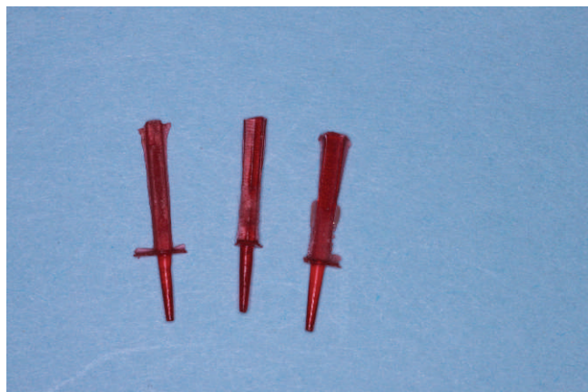
Figure 8. Plastic burnout pins used for vent pin.
