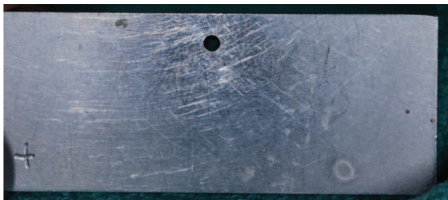
Figure 3. The stainless steel block with the tapered space to form the resin pattern to be cast.
