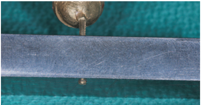
Figure 5. The casting tried back in the steel block after examination to ensure no nodules are present on the casting. If the casting is smaller, it will pass through the channel, and the tip will protrude out the inferior border of the steel block. The length of the post is measured from the tip of the post to the border of the steel block.
