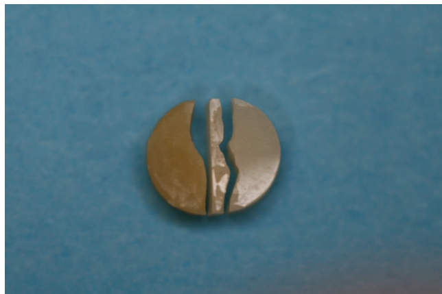
Figure 1. Diametral tensile failure. The fracture occurred along the repair site and through adjacent composite resin. This is referred to as a cleft fracture and was classified as a mixed fracture.
