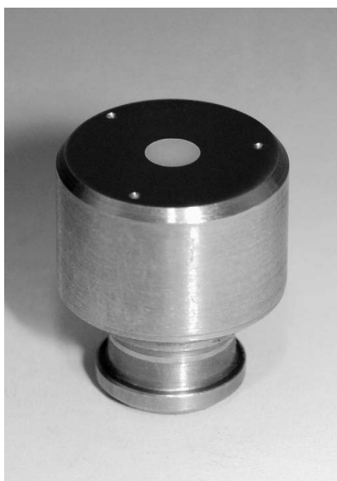
Figure 2. Stainless steel custom fixture for generalized wear.
