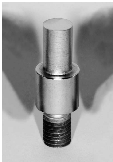
Figure 4. Stainless steel antagonist tip for simulated generalized wear.
