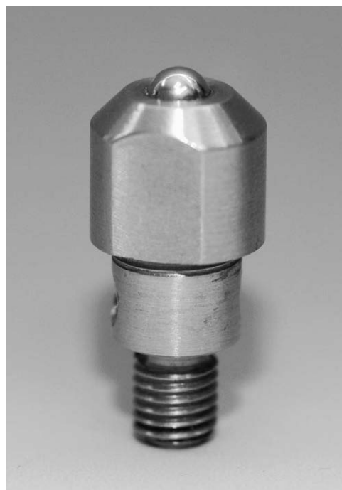
Figure 3. Stainless steel antagonist tip for simulated localized wear.
