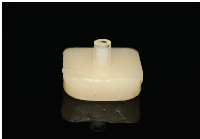
Figure 1. Composite tube affixed to the coupon of lithium disilicate.
