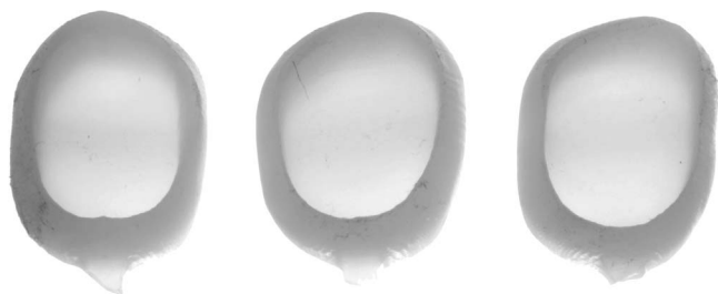
Figure 6. Translucency confirming homogenous material thickness within specimens.
