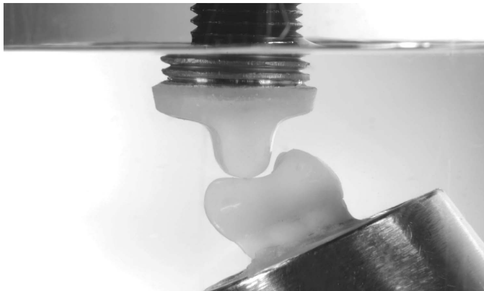
Figure 3. Specimen in load chamber, filled with distilled water to submerge specimen during testing.
