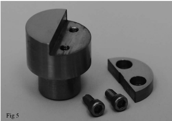
Figure 4. Slit (gap) fixture for generalized wear simulation.
