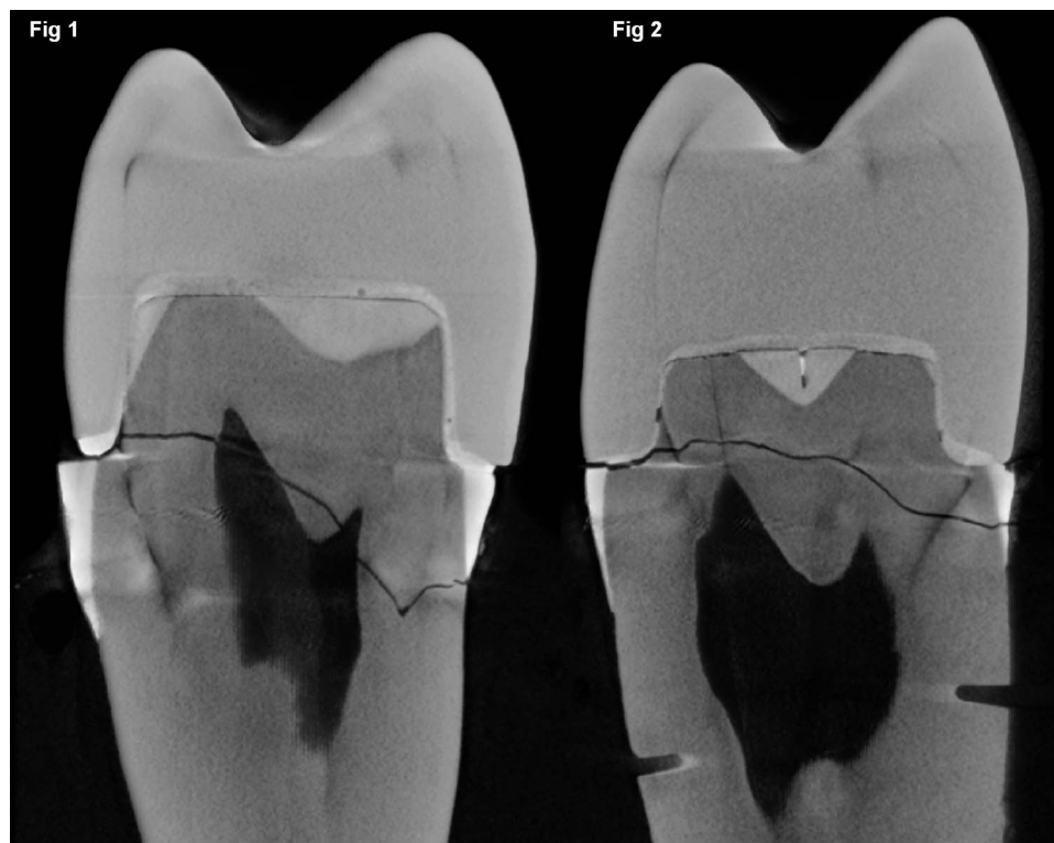
Figure 1. MicroCT image slice showing 3-mm occlusocervical axial height failure.
