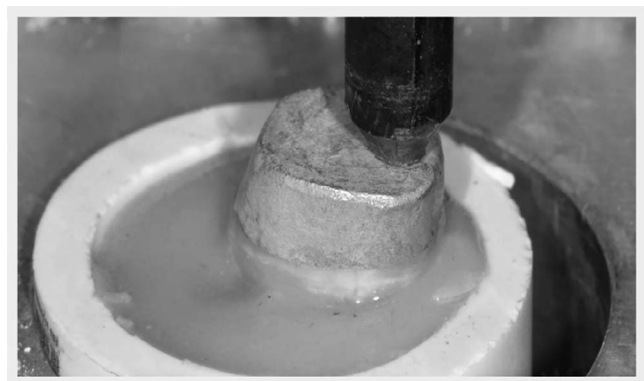
Figure 3. The specimens were removed from the typodont and mounted in polyvinyl chloride pipe. After 24 hours of storage, the specimens were mounted in a universal testing machine. A round-ended blade was lowered onto the marginal ridge. The mean maximum force in newtons and standard deviation were determined per group (n=10).
