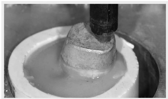
Figure 3. The specimens were removed from the typodont and mounted in polyvinyl chloride pipe. After 24 hours of storage, the specimens were mounted in a universal testing machine. A round-ended blade was lowered onto the marginal ridge. The mean maximum force in newtons and standard deviation were determined per group (n=10).
