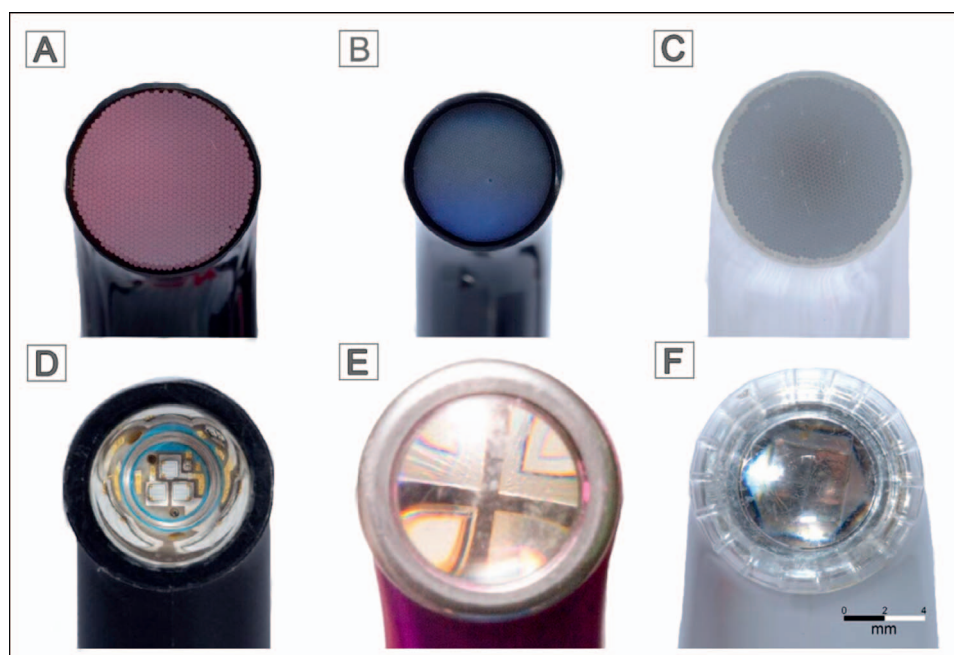
Figure 2. LED light-curing tips. (A): Bluephase Style. (B): ESPE Cordless. (C): Elipar S10. (D): Demi Ultra. (E): Valo Cordless. (F): Radii-Cal. Note the different tip diameters (all tips imaged to the same mm scale).
