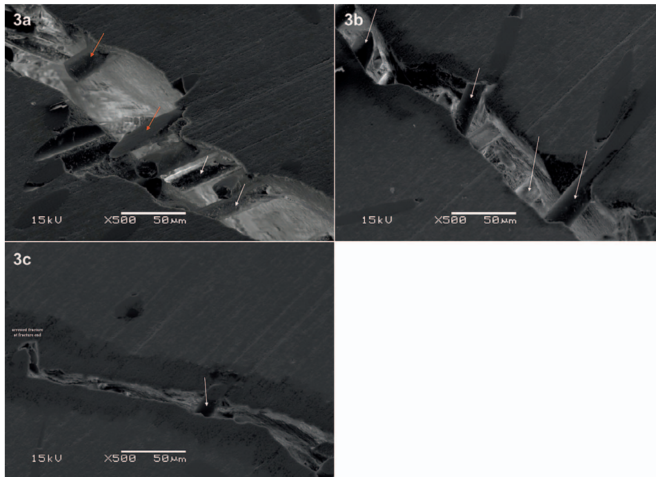
Figure 3. (a-c): SEM micrographs showing typical fracture line segments. (a): SEM micrograph (500×) showing protruding fibers at the interface (red arrows) and bridging fibers (white arrows) at the beginning of the fracture line (near the notch). (b): SEM micrograph (500×) showing bridging fibers (white arrows) at the middle part of the fracture line. (c): SEM micrograph (500×) showing bridging fibers (white arrows) at the end part of the arrested fracture line.
