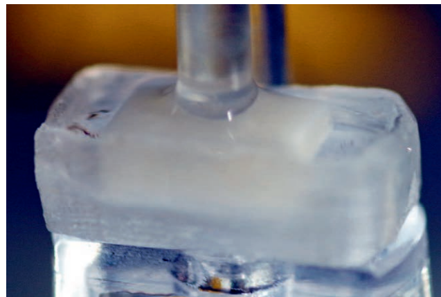
Figure 1. Quartz container on TMA platform showing immersed sample.
