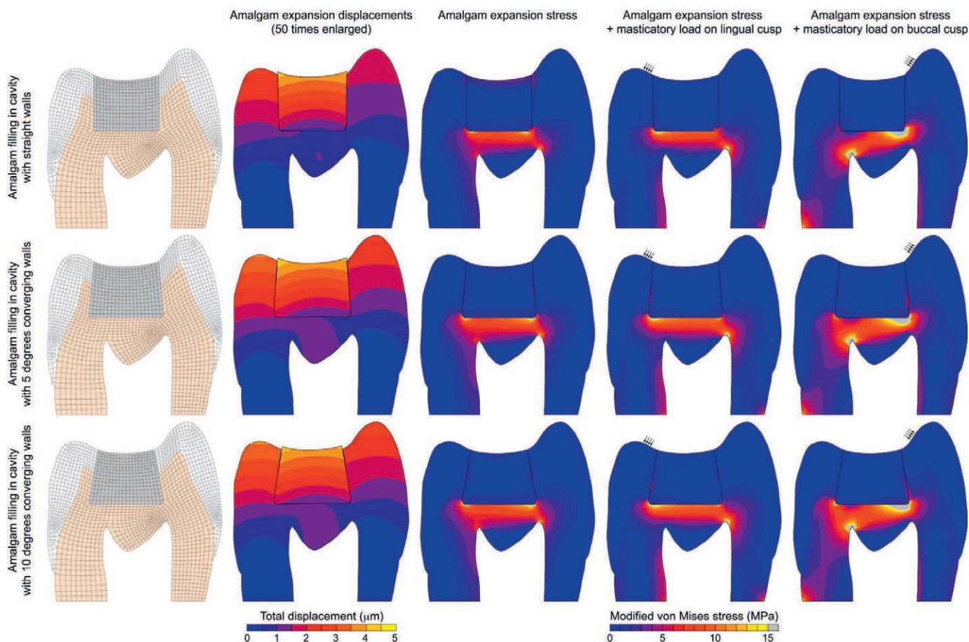
Figure 3. Calculated displacements and stresses in the cross section of an amalgam-filled tooth with 3- \mu m cuspal flexure due to amalgam expansion. Stress concentrations are seen at the cavity line angles. Stress concentrations intensified when a masticatory load was added on the lingual or buccal cusp (20 N over 1.5 mm 2 area, indicated with arrows).
