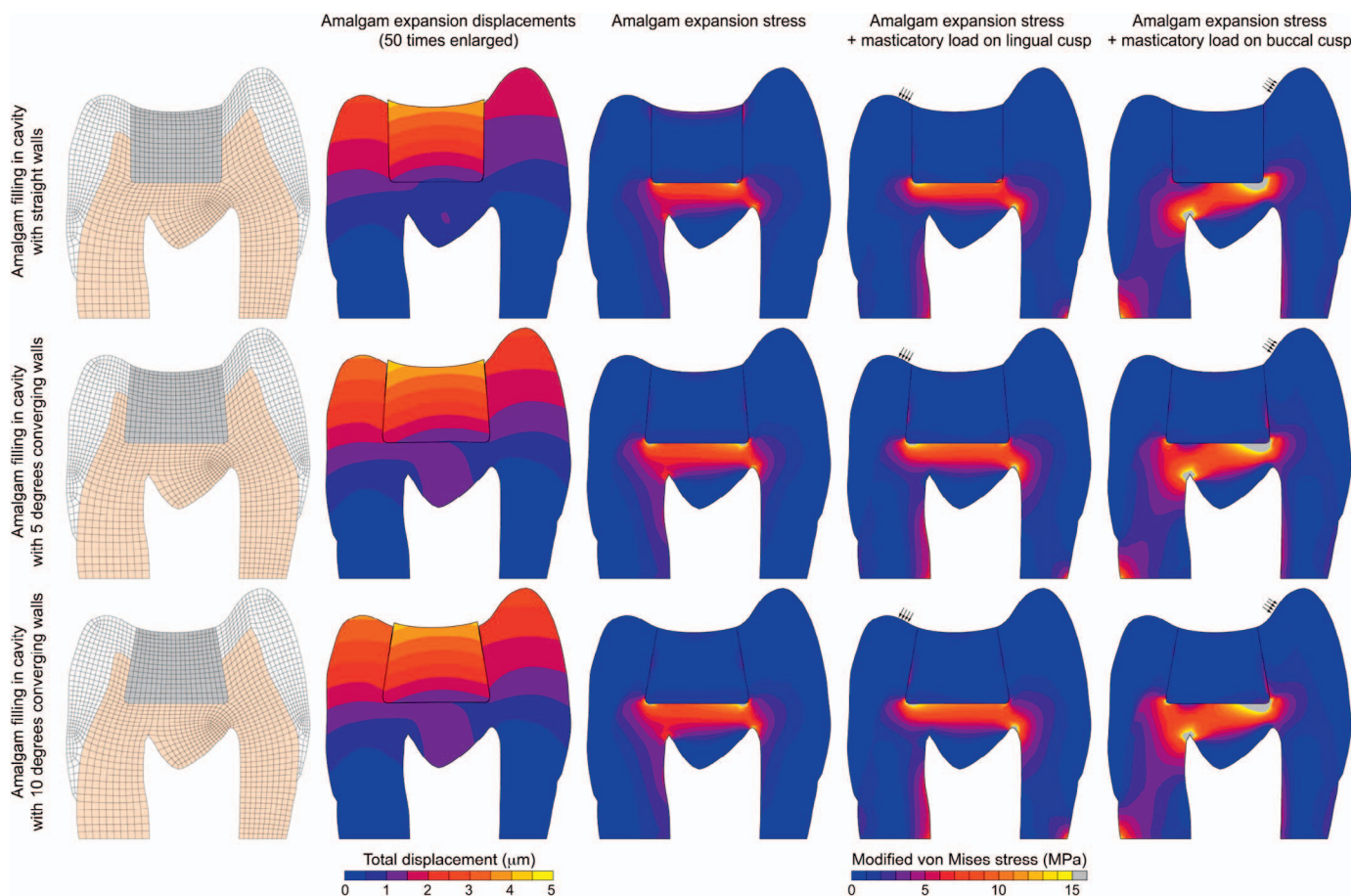
Figure 3. Calculated displacements and stresses in the cross section of an amalgam-filled tooth with 3- \mu\text{m} cuspal flexure due to amalgam expansion. Stress concentrations are seen at the cavity line angles. Stress concentrations intensified when a masticatory load was added on the lingual or buccal cusp (20 N over 1.5 mm 2 area, indicated with arrows).
