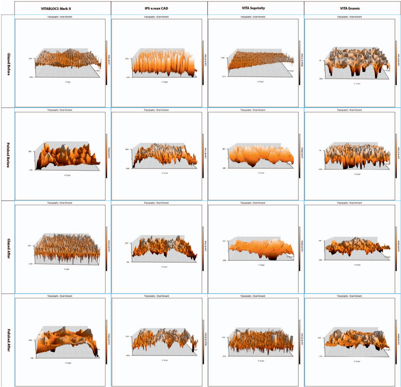
Figure 1. Ceramic roughness measurement before and after the wear test by AFM (Ra).
