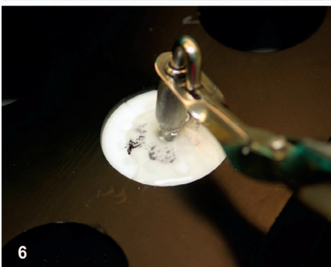
Figure 5. Within the 3.5 mm-diameter specimen wells, the 1.5 mm-diameter condenser tip was placed once in the center and eight times around the perimeter to provide thorough condensation.
