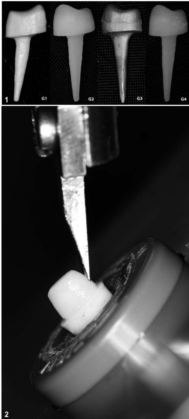
Figure 1. Representative customized post-and-core from each group. G1, specimen (PEEK post-and-core); G2, specimen (nano-ceramic composite [Lava Ultimate] post-and core); G3, specimen (metal cast post-and core); G4, specimen (fiberglass customized with nano-hybrid resin composite post-and core).
